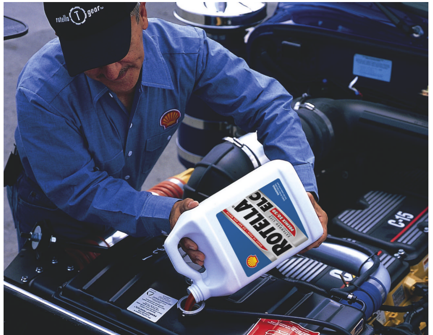
When using extended life coolant, it is critical that you top off the coolant level, as shown here, with the proper ELC coolant additive. OEMs do not recommend mixing ELC with conventional coolants. Photo courtesy of Shell Rotella
