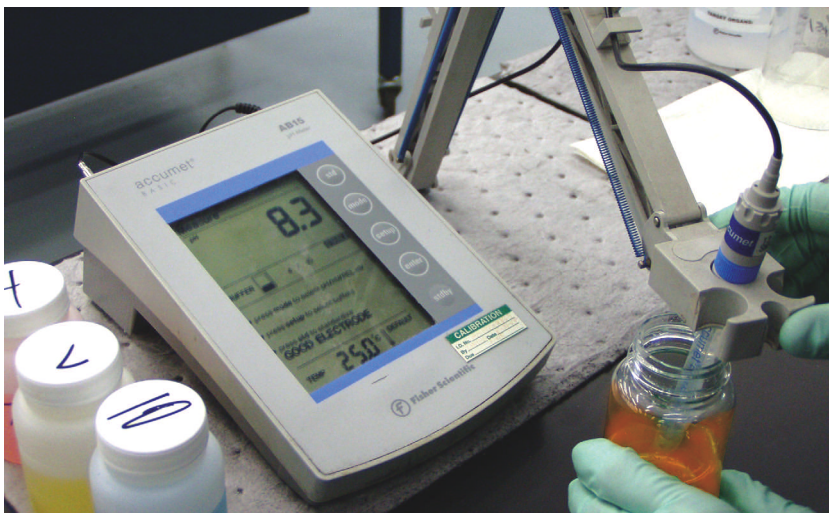
Laboratory equipment, such as this at Polaris Laboratories, is used to test for conductivity and total dissolved solids (TDS) in coolant samples.
